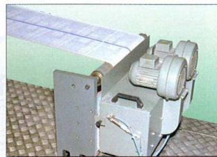
UV-dryer, 520 mm, 10 kW for endless paper press.
