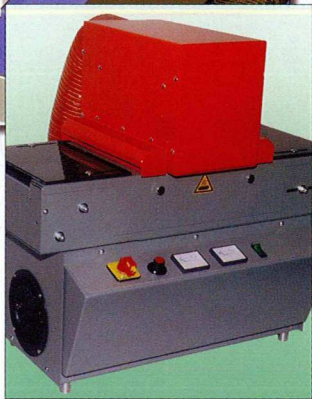
UV-belt conveyor 150 mm, 2 KW
