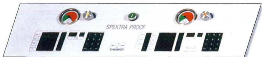
User panel with vacuum meter, switch for 3 power levels, KR-Computer and LED display
